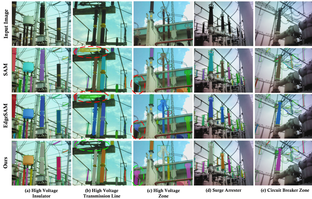
Figure 6: Some examples of segmentation results are shown with the results of SAMs in the second and third lines and our proposed method in the fourth line. The original images are shown on the top line. Several examples show that our proposed method can better segment the substation equipment in complex scenes.
